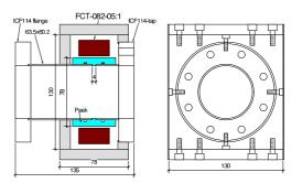
Fig. 2. Mechanical drawing of FCT monitor housing
