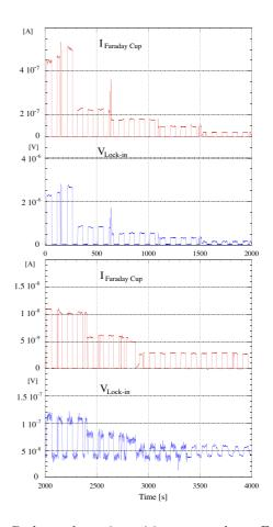
Fig. 4. Cyclotron beam intensities measured at a Faraday cup and voltages of the lock-in amplifier for various intensities. The time constant for the lock-in amplifier was 300 ms except for the last 5 peaks which were at 1 s (3 peaks) and 3 s (2 peaks).
