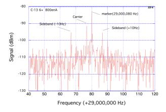
Fig. 3. Power spectrum of the second harmonics of 100A-MeV  $^{13}\mathrm{C}^{6+}$  beam of 800 enA detected by FCT. Sidebands due to a chopped beam with 10 Hz as well as the carrier signal at  ${\sim}29$  MHz are observed.
