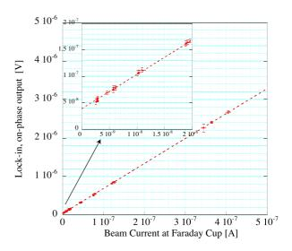
Fig. 5. 'On-phase' voltage of lock-in amplifier signal vs. beam current measured at Faraday cup. Insert is an enlarged graph for lower intensities. The fitting line is  $y = 6.49(4) \cdot x + 39(1) \times 10^{-9}$
