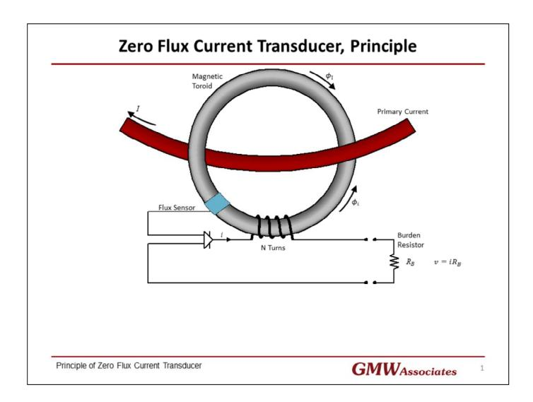
The primary current, I, in a conductor through a magnetic core will generate a magnetic flux in the core  $\phi_I$ . If somehow this flux in the core can be sensed by a "core flux sensor" then a compensation current, i, in a winding around the core can be used to generate an opposite flux  $\phi_i$  so that  $\phi_i = \phi_I$ . The compensation current, I, can be measured in a "Burden Resistor"  $R_B$  as  $v = I \cdot R_B$ .
