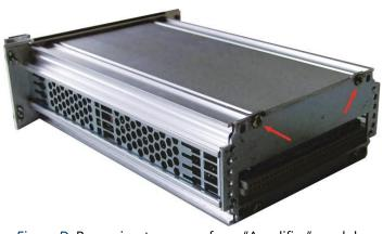
Figure D: Removing top cover from "Amplifier" module.
