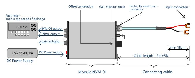
Figure 1: Typical measurement setup with a SENIS NVM-01
