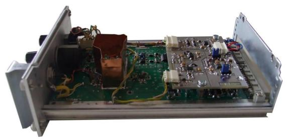
Figure E: Amplifier module without top cover.
