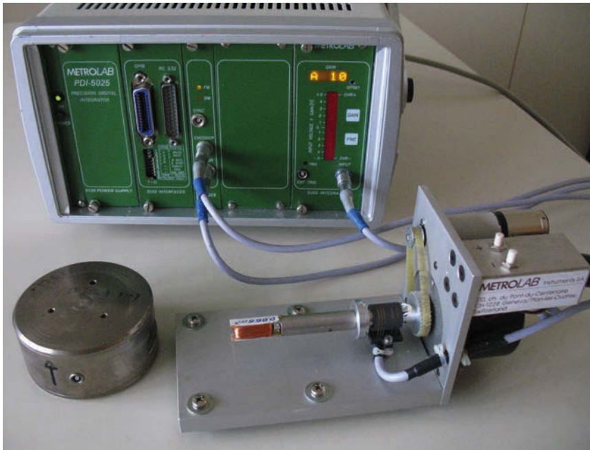
Figure 3: Scale model of the setup used by physicists to characterize particle beam magnets. A long rotating coil measures the integrated field seen by the particle beam – which determines the kick – as a function of angle. The Fourier transform of these angular measurements yield the components relevant for the beam optics. For example, a dipole magnet, which steers the beam, generates a single sinusoidal period per coil rotation, whereas a quadrupole, which focuses/defocuses the beam, generates two periods. Real magnets, for example a quadrupole whose poles are not perfectly matched, generate some mix of these and higher-order components. Clockwise from the top: PDI5025 voltage integrator, rotating-coil jig with angular encoder, and the magnet under test
