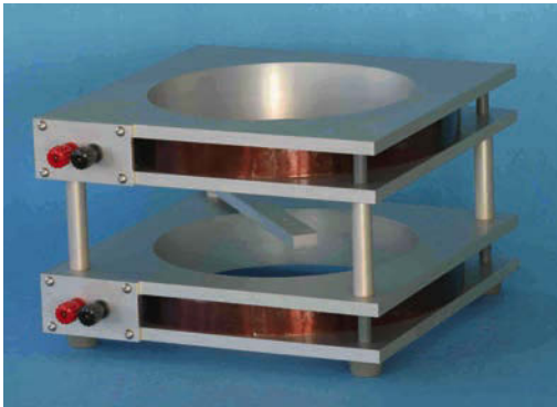
Figure 2 (left and below): An example of a modern-day industrial fluxmeter, with a Helmholtz coil to measure the magnetic dipole of permanent magnets. Images courtesy of Magnet-Physik Dr SteinGroever, Cologne, Germany
