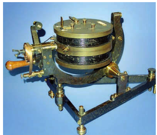
Figure 1 (right and below right): The flip-coil and the ballistic galvanometer, a classic fluxmeter. Images courtesy of the Historical Scientific Instrument Gallery, Department of Physics, University of Nebraska
