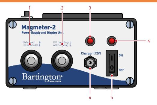
Figure 1. Magmeter-2 Front Panel
