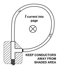
The sensitivity of the CWT to currents that do not pass through the coil is very small, provided that such currents are no greater than the CWT's rating or such currents are relatively distant from the coil. In the vicinity of a multi-turn inductor the 'H' field is far stronger than from a single conductor carrying the same current, and such positions should be avoided.
