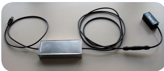
Figure 3. Prototype of the THM1176 electronics with a Bartington Mag649. The only required modification was the addition of differential receivers.
