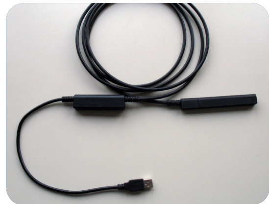
Figure 2. The complete magnetometer. The probe with the sensor is connected to a small dangle containing the instrument electronics, which in turn is powered and controlled via USB.
