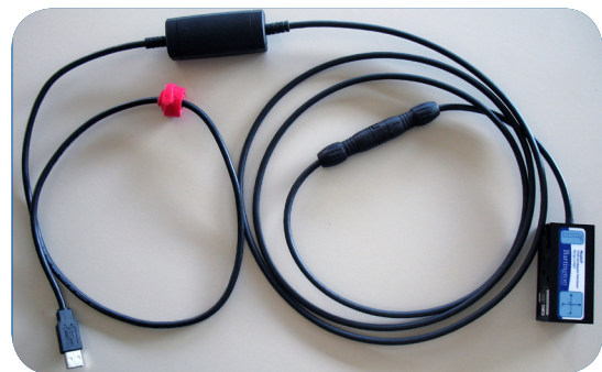
Figure 4. Metrolab’s Three-axis Fluxgate Magnetometer, TFM1186. For simplicity, the differential receivers are on a second PCB, requiring a slightly larger housing than for the THM1176.
