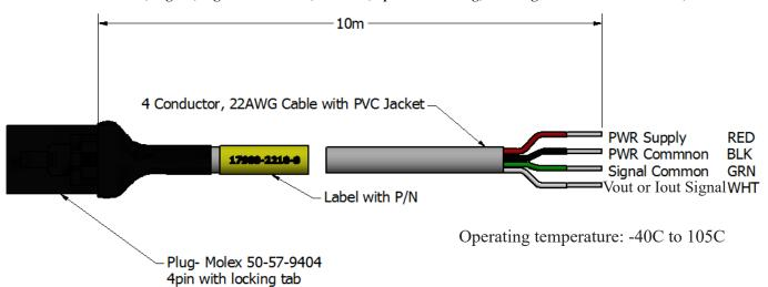
17900-2211-0 Cable, Pigtail, Signal and Power, 22AWG, 4pin Molex Plug, Locking tab and Unterminated, PVC Jacket, 1m
