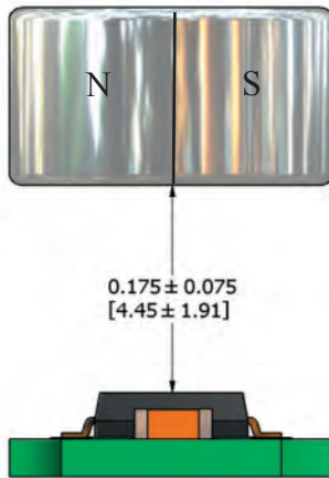
Air Gap Operating Range for the 55B0082 Cylindrical Magnet
