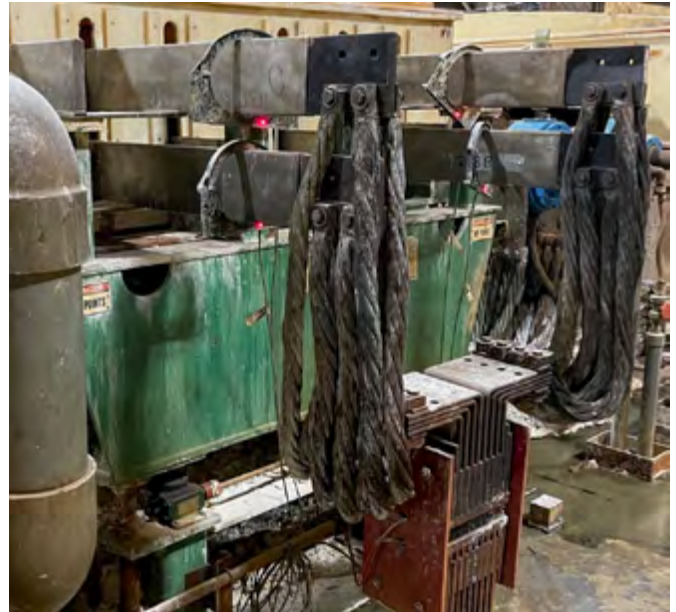
Figure 4: Four CPO Clamp-On, 160mm aperture, 12kA Current Probes used to monitor bus bar current in an electrochemical application with reliable operation in a harsh environment.
