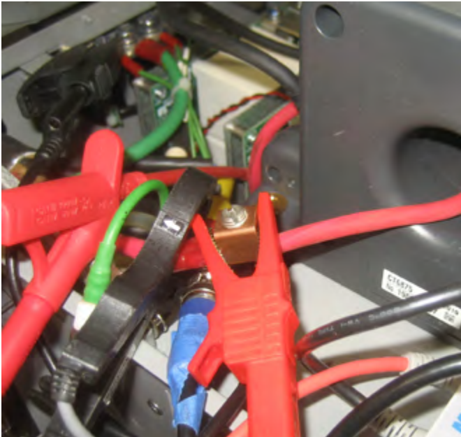
Figure 3: The very small size of the CPC Current Probe Clip enables it to be used in parallel with a Rogowski Coil to measure dc and low frequency current components on a vehicle charging cable without disconnection of any cables. Courtesy Argonne National Laboratory, Ted Bohn.
