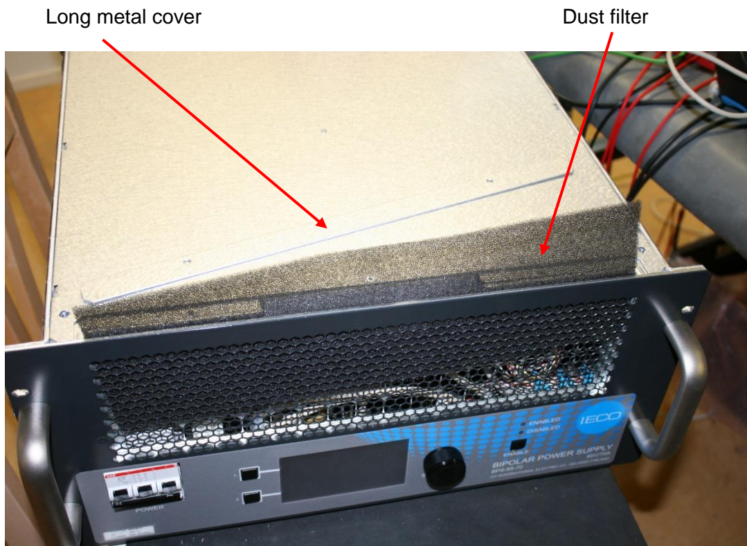
Figure 23: Dust filter replacement
