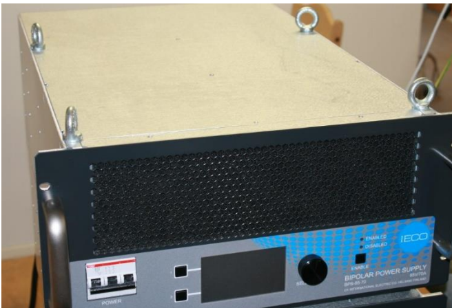
Figure 4: Lifting eyes at roof of BPS
