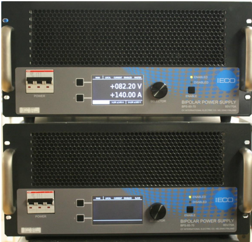
Figure 22: Parallel operation in use.
