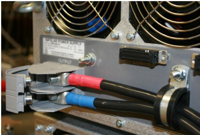
Figure 10: Output terminal and cables. Cable tie is not shown in picture.
